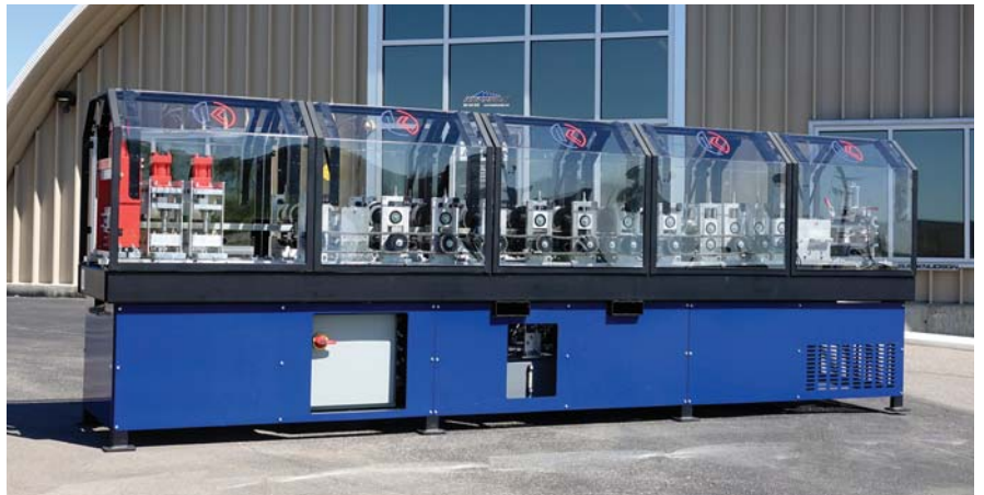
KFS-1622E Structural Stud and Track Forming Machine from Knudson Mfg.
